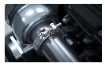
**V-Band clamps** are ideal for applications in which the exhaust gas temperature range is up to 650 °C - for example, in diesel engines and heavy-duty vehicles.
